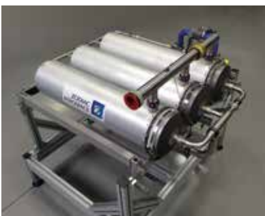
(1) On-Board Inerting Gas Generating System.
