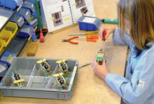
The power contactors assembly shop for electrical power distribution systems at the Niort plant.
