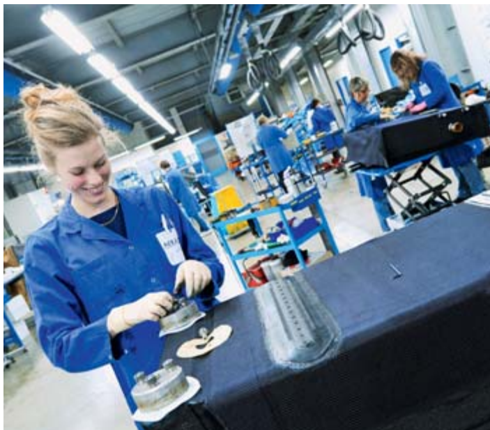
Building an anti-crash tank for the Super Puma AS332 helicopters.
